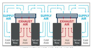
ALTERNATING HOT AND COLD AISLES provide efficient air segregation
