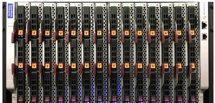
14 disaggregated servers in a 6U blade chassis with integrated network switch
