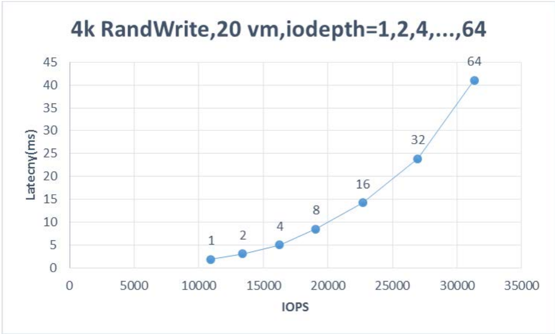
Figure 8. Random Write IOPS and Latency on a 4-node VirtualStor™ Scaler Cluster.
